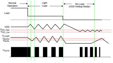
Figure 3. Burst Triple Mode
